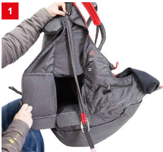
Connect the rescue bridles to the rescue riser
