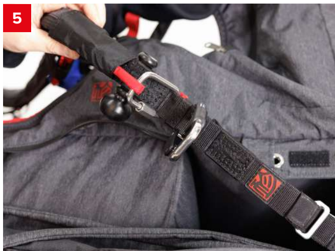
Close the velcro panel of the spreader bar
