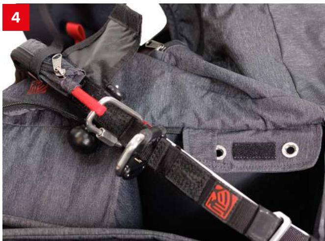
Connect the rescue bridle to the spreader maillon and close it.
